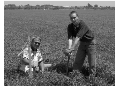
District Technician Sean Brown (right), installs a tensiometer with land owner Paul Schlagel as part of an irrigation management system.
